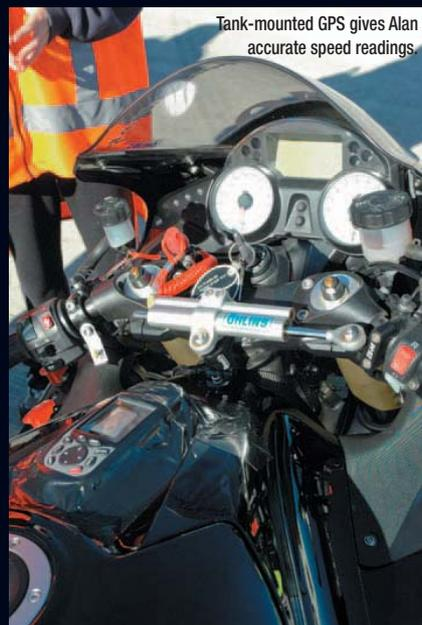
Tank-mounted GPS gives Alan accurate speed readings.
